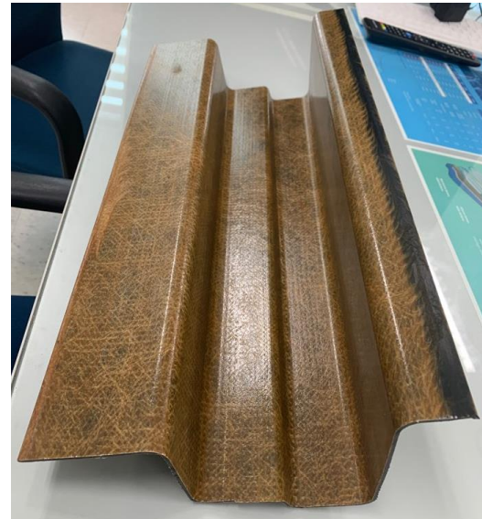
Carbon/Glass Hybrid structure
